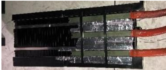
Figure 4-4: Ignition heater layout along bottom of module.
