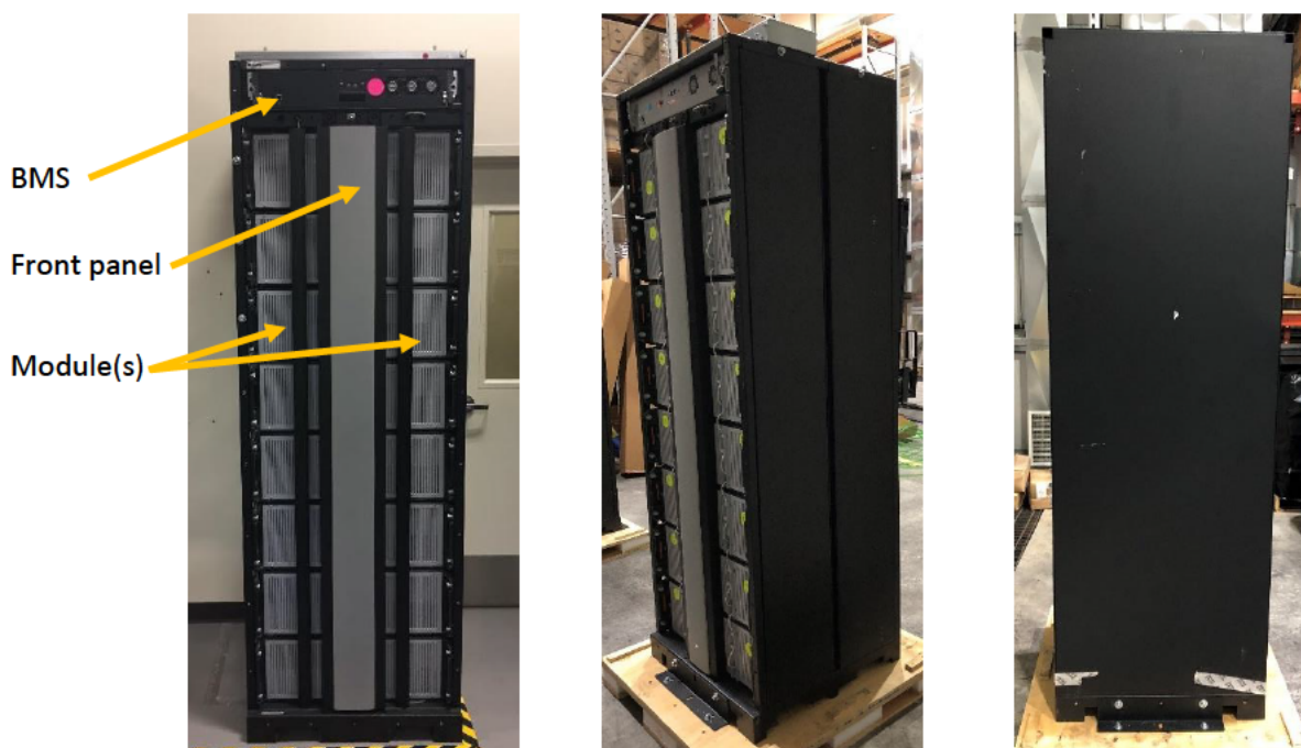
Figure 3-3: Photos of LNO/LMO rack; front (right), side (middle), and back (right).
