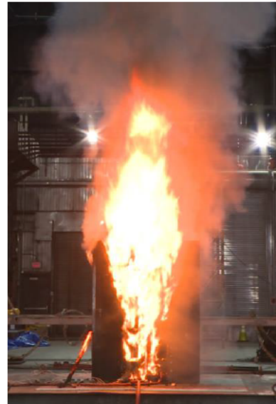
Figure A-1: Left panel: a plan view of test configuration, (not to scale); right panel: fire image of Li-ion battery fire test.
