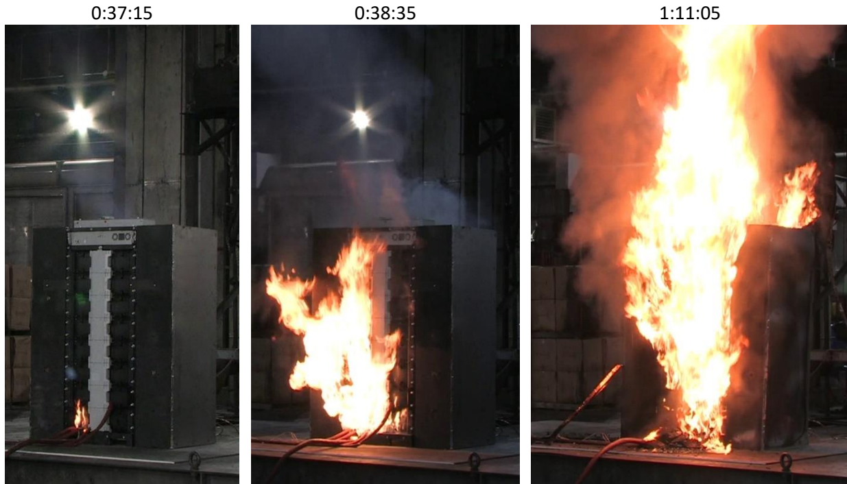
Figure 6-3: Photos of LFP fire development during large-scale free burn test: near time of ignition (left), near time of predicted sprinkler operation (middle), peak heat release rate (right).
